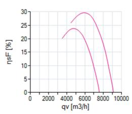
measured in full bell mouth without guard grille in installation type A according to ISO 5801 Please note: It's not allowed to use this fan in the stall area!\*
